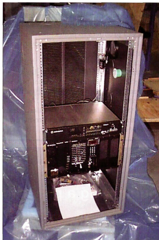
FIGURE 8. A large piece of telecommunications equipment that was being packaged for shipment utilizing VCI technology.
